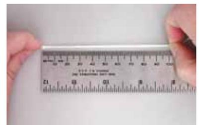
After measuring a root, placing the string next to a ruler to calculate the actual root length.
